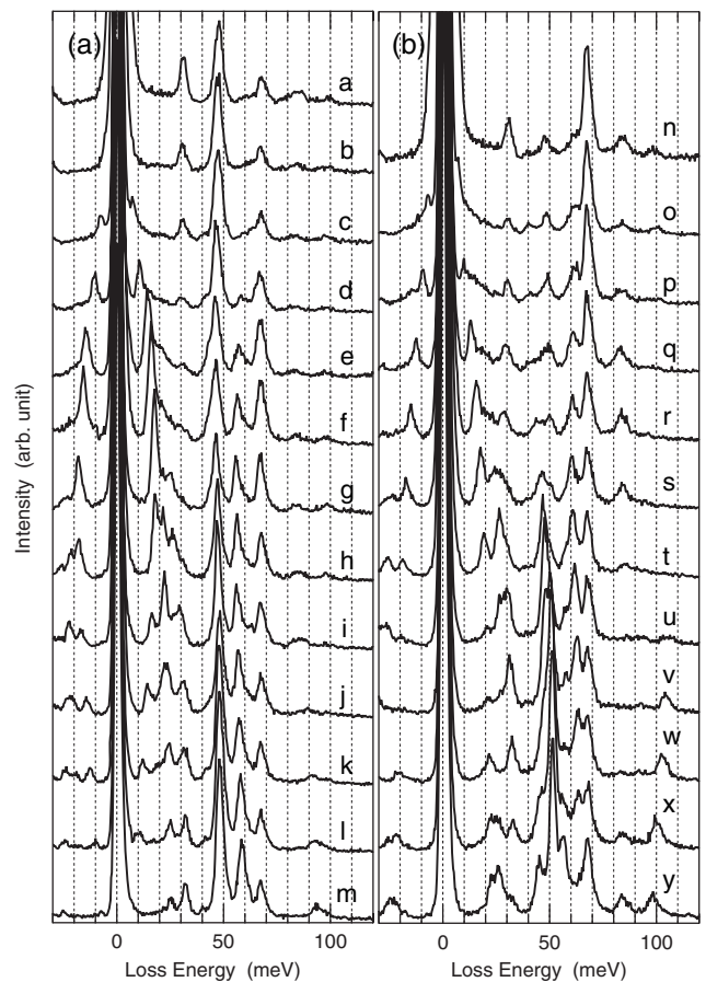
Figure 3. Series of off-specular HR-EELS spectra along (a) [11\bar{2}0] ( \bar{\Gamma}-\bar{M}-\bar{\Gamma} ) and (b) [10\bar{1}0] ( \bar{\Gamma}-\bar{K}-\bar{M} ) directions. The primary electron energy is 22.1 eV and the incidence angle is 75^\circ from the surface normal. The detection angles from the surface normal are a: 69.4^\circ , b: 64.9^\circ , c: 60.3^\circ , d: 55.7^\circ , e: 51.1^\circ , f: 47.7^\circ , g: 44.2^\circ , h: 40.8^\circ , i: 37.3^\circ , j: 35.0^\circ , k: 32.8^\circ , l: 30.5^\circ , m: 28.2^\circ , n: 68.3^\circ , o: 62.6^\circ , p: 58.0^\circ , q: 53.4^\circ , r: 50.0^\circ , s: 46.5^\circ , t: 43.1^\circ , u: 39.6^\circ , v: 36.4^\circ , w: 33.2^\circ , x: 30.2^\circ , and y: 27.2^\circ .
